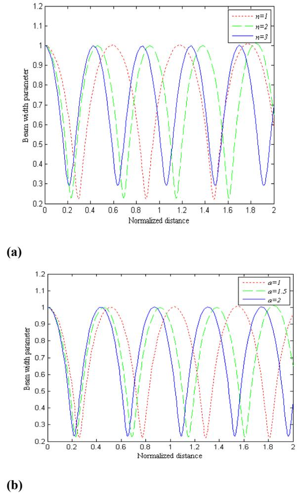
**Figure 1.** Variation of beam width parameter ( $f_0$ ) of hollow Gaussian laser beam with normalized propagation distance ( $\xi$ ): (a) for different orders of HGB ( $n = 1, 2$  and  $3$ ) with  $a = 1.5$  and  $\omega_{p0} = 0.3\omega_0$  (b) for different values of  $a$  ( $= 1, 1.5$  and  $2$ ) with  $n = 2$  and  $\omega_{p0} = 0.3\omega_0$ , when both relativistic and ponderomotive nonlinearities are operative.
