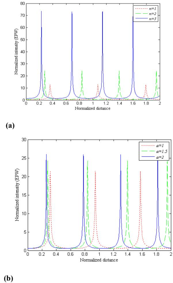
**Figure 3.** Variation in normalized intensity of EPW with normalized distance of propagation ( $\zeta$ ): **(a)** for various orders of HGB ( $n = 1, 2$  and  $3$ ) with  $a = 1.5$  and  $\omega_{p0} = 0.3\omega_0$  **(b)** for different values of  $a$  ( $=1, 1.5, 2$ ) with  $n = 2$  and  $\omega_{p0} = 0.3\omega_0$  and , when both relativistic and ponderomotive nonlinearities are taken into account.
