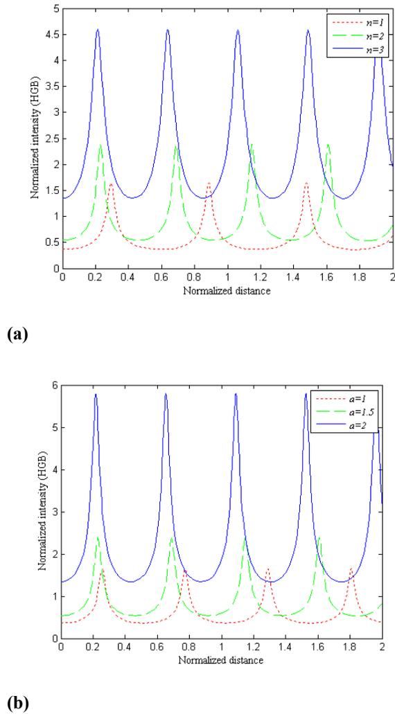
**Figure 2.** Variation of normalized laser beam intensity in plasma with normalized distance of propagation ( $\zeta$ ): **(a)** for different orders of HGB ( $n = 1, 2$  and  $3$ ) with  $a = 1.5$  and  $\omega_{p0} = 0.3\omega_0$  **(b)** for different values of  $a$  ( $=1, 1.5$  and  $2$ ) with  $n = 2$  and  $\omega_{p0} = 0.3\omega_0$ , when both relativistic and ponderomotive nonlinearities are operative.
