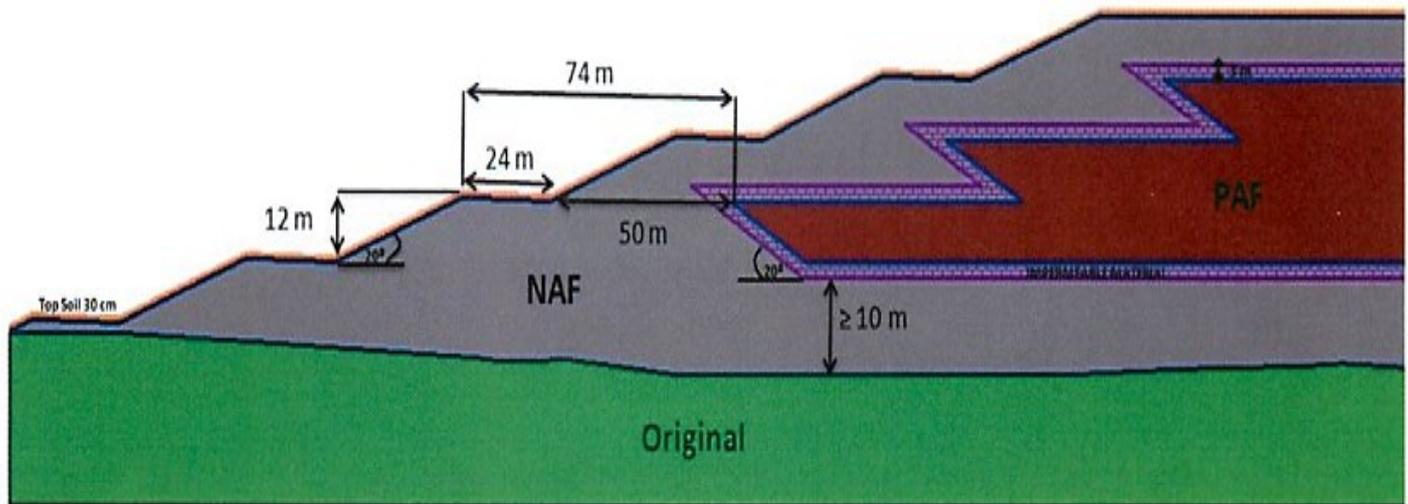
FIGURE 6. Cross Section of Disposal Design
